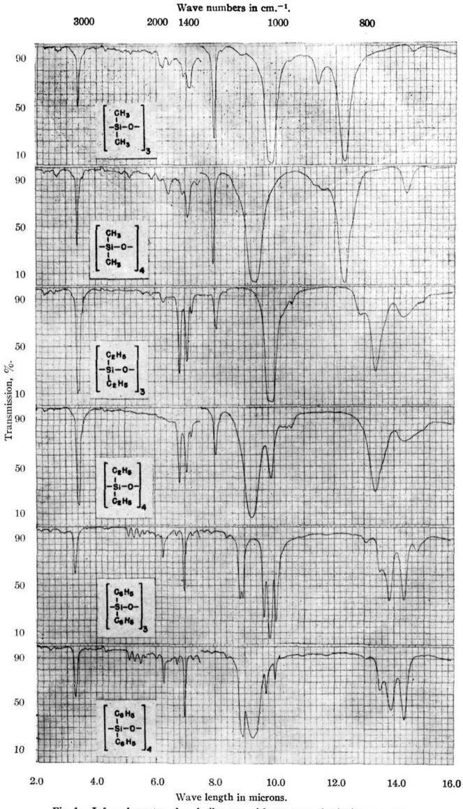
Fig. 1.--Infrared spectra of cyclosiloxanes with one type of substituent group.
